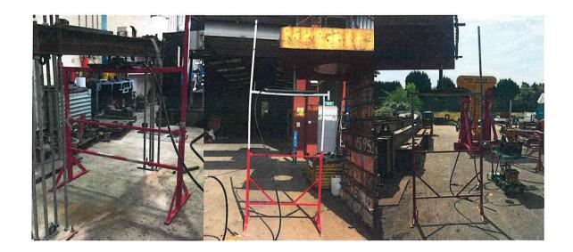
BS1139 Part 4 1982 requires that each stand should be able to withstand 2 ½ times the stated SWL without failure at 1°30 out of plumb without ultimate failure. The test load was applied as per the code, each load point to be 75mm at 1/4 span in from each end.
